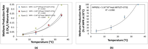
Figure 4. Average methane production rate (a) and the average methane production rate as percent of the rate at 35°C (b) as a function of temperature with the fitted Arrhenius equation.
