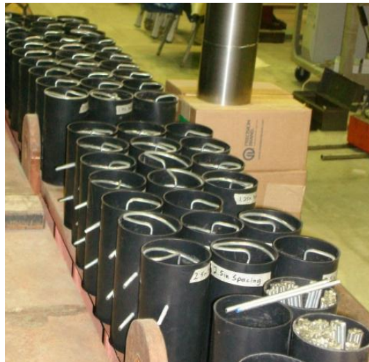
Figure 5-4: Constructed concrete cylinder molds prior to placement of concrete
