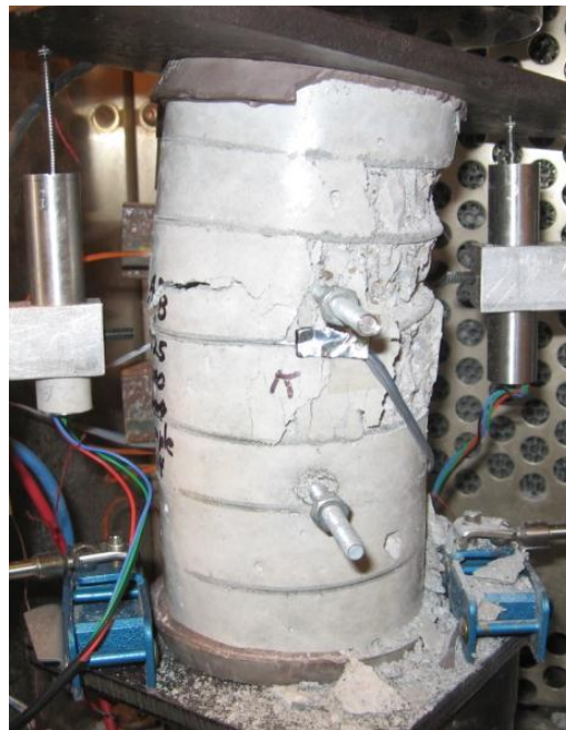
Figure 5-6: Axial and bending failure of confined concrete cylinder when upper head rotated after damage to the confined specimen
