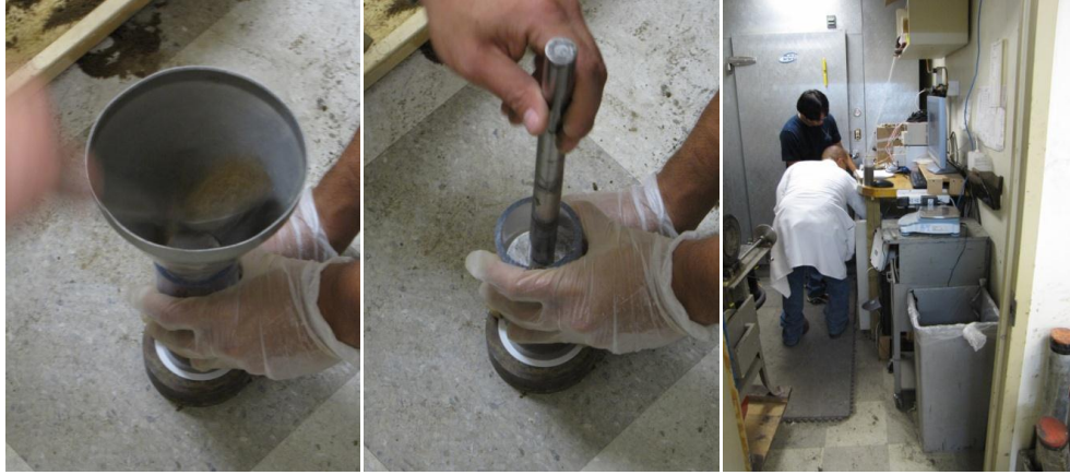
Figure 7-1: Sample compaction process: (a) loosely placing soil in mold; (b) using a plunger to compact soil; (c) placing compacted soil and molds in storage freezer
