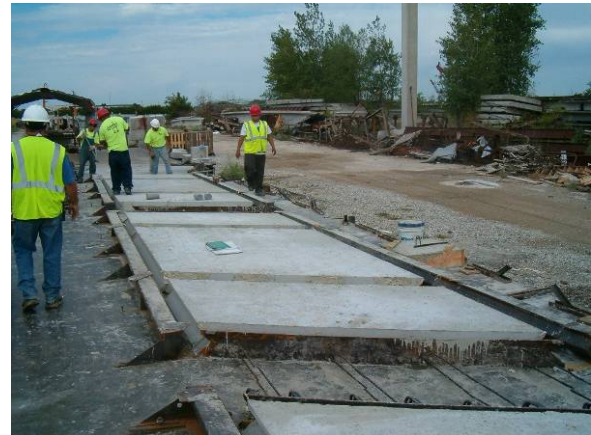
Figure 2. Panel form release
