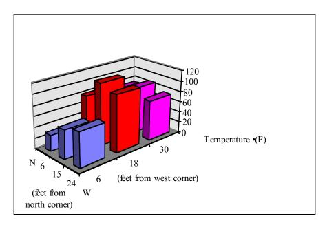
Figure 2. Average temperatures at various locations in the bedded pack of a hoop structure (Rhodes Farm, 2/27/97).
