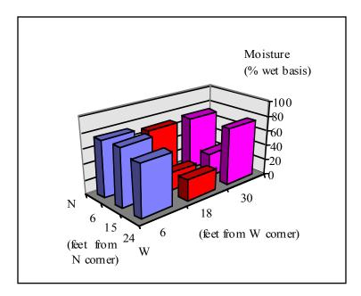
Figure 3. Moisture variation in the bedded pack of a hoop structure (Rhodes Farm, 2/27/97).
