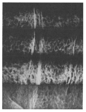
Fig. 8. Enlarged view of linear arrays in the montage of gallium arsenide topographs.
