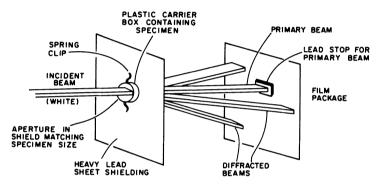
Fig. 2. Schematic for white beam transmission topography.
