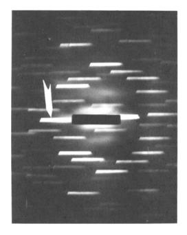
Fig. 3. Full size (8 x 10 inch) topograph of gallium arsenide substrate.
