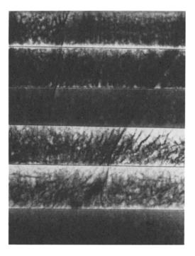
Fig. 7. A different section of the montage of topographs of gallium arsenide. Note the large linear arrays.
