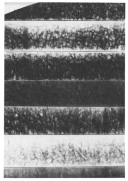
Fig. 6. A section of the montage of topographs of gallium arsenide. Note the outer edge of the three inch diameter substrate at upper left.
