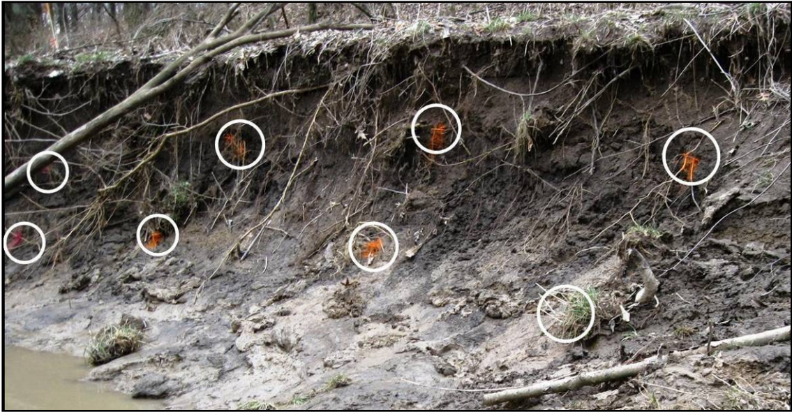
Figure 9. Photo of erosion pin placement on a stream that is between 1-2 m tall.
