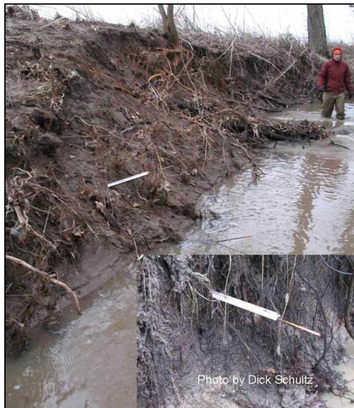
Figure 7. Photos of severely to very severely eroding banks. The orange pole (A) represents the downstream end of a pin plot. The ruler (B) is 30 cm long and is used when measuring pins.
