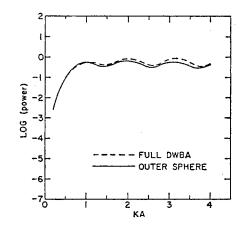
ig. 2. Spherical cavity in Ti: Longitudinal backscattered wave, log (power) versus ka for a ratio of radii of 6/5.
