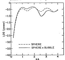
Fig. 11. Bubble defect in Ti: Longitudinal backscattered wave, log (power) versus ka for incidence direction  $\theta_0 = 90$ .
