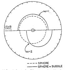
Fig. 16. Bubble defect in Ti: Longitudinal wave, log (power) versus azimuthal angle  $\phi$  for incidence direction  $\theta_0 = 90$ , scattering angle  $\theta = 135$ , and ka = 1,2. SUMMARY
