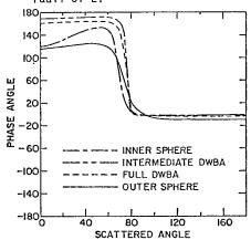
Fig. 8. Al sphere in Ti: Longitudinal wave, phase angle versus 0 for ka = 1 and ratio of radii of 2.
