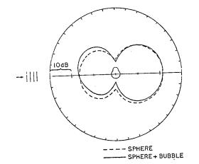
Fig. 15. Bubble defect in Ti: Longitudinal wave, log (power) versus scattering angle  $\theta$  for incident direction  $\theta_0 = 90$ , ka = 2; the scattered direction is in the plane defined by the incident direction and the symmetry axis of the scatterer.
