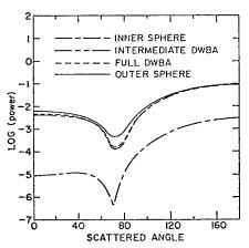
Fig. 7. Al sphere in Ti: Longitudinal wave, log (power) versus θ for ka = 1 and ratio of radii of 2.
