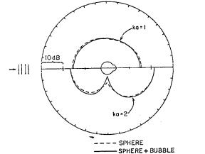
Fig. 13. Bubble defect in Ti: Longitudinal wave, log (power) versus θ for shadowed incidence, ka = 1,2.
