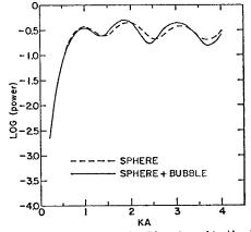
Fig. 10. Bubble defect in Ti: Longitudinal backscattered power, log (power) versus ka for shadowed incidence,  $\theta_0 = 0$ .
