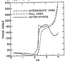
Fig. 6. Al sphere in Ti: Longitudinal backscattered wave, phase angle versus ka for a ratio of radii of 2.
