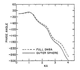
Fig. 3. Spherical cavity in Ti: Longitudinal backscattered wave, phase angle versus ka for a ratio of radii of 6/5.
