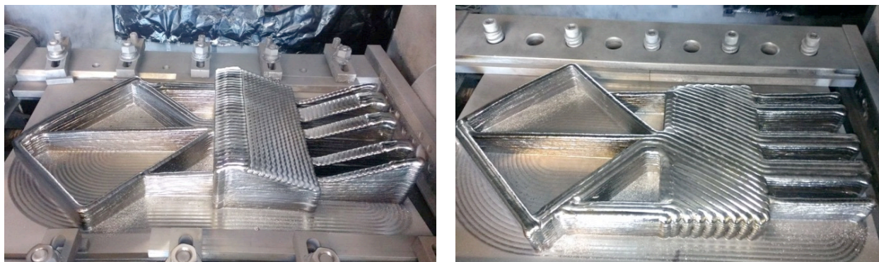
Figure 1. Electron beam additive manufacturing notional part; top (left) and bottom (right).
