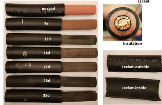
FIGURE 6. EPR/TS-CPE cable samples aged at 140°C for up to 35 d in 7 d increments. After aging, part of the jacket was removed.
