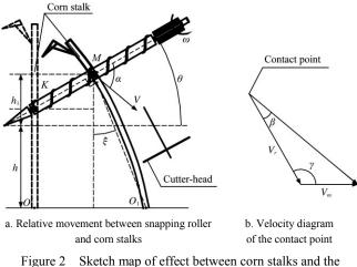
Figure 2 Sketch map of effect between corn stalks and the snapping roller
