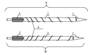
A. Outer snapping roller B. Inner snapping roller 1. Tapering portion
