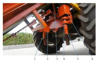
Cutter-head 2. Adjust mechanism of cutting angle 3. Driving chain
