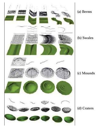
Figure 7: Generic subset of topographic primitives, abstracted as blades and paths shapes
