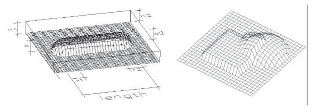
Figure 8. A parameterized berm primitive left.
