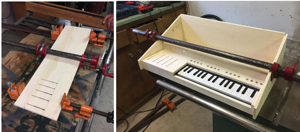
Figure 16: Gain Slit Panel Construction and Body Construction
