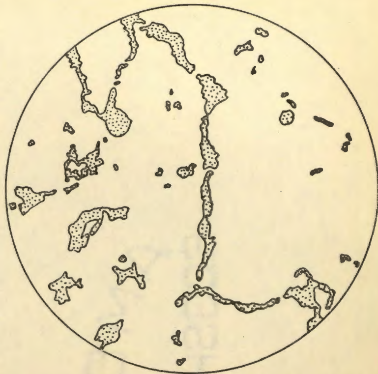
FIG. 4. Microprojection tracing. Surface horizon, Shelby silt loam. Stippled areas represent pore space. 44.5 \times .
