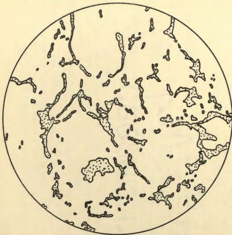
FIG. 9. Microprojection tracing. Surface horizon (virgin), Marshall silt loam. Stippled areas represent pore space. 44.5 \times .
