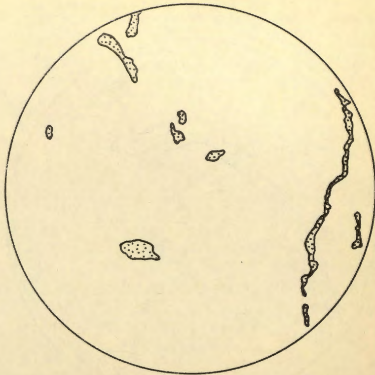
FIG. 8. Microprojection tracing. C-29 inch horizon, Shelby silt loam. Stippled areas represent pore space. 44.5 \times .
