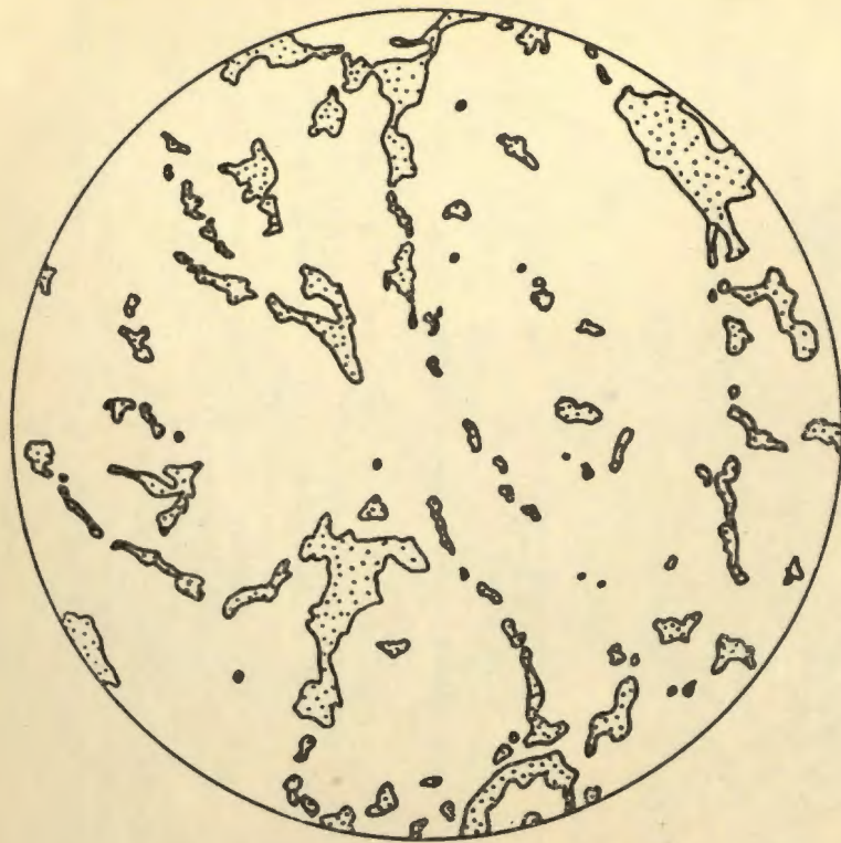
FIG. 3. Microprojection tracing. Surface horizon, Marshall silt loam. Stippled areas represent pore space. 44.5 \times .
