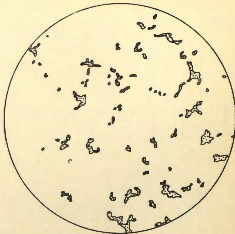
FIG. 10. Microprojection tracing. Surface horizon (cultivated), Marshall silt loam. Stippled areas represent pore space. 44.5 \times .
