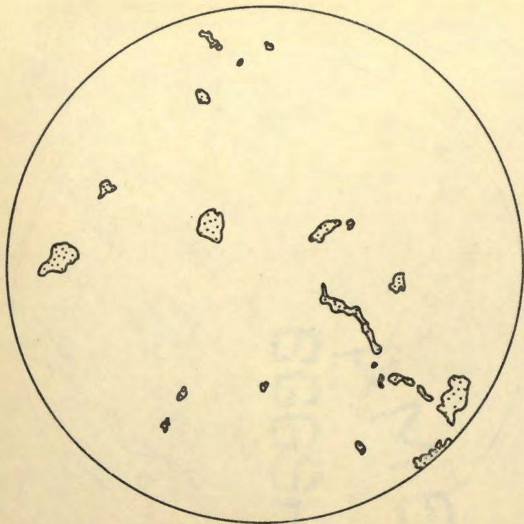
FIG. 7. Microprojection tracing. C-40 inch horizon, Marshall silt loam. Stippled areas represent pore space. 44.5 \times .
