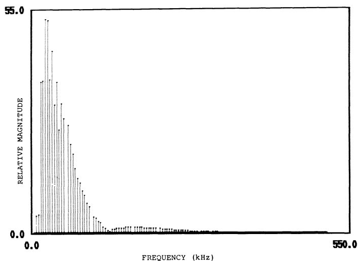
Figure 4—Frequency spectrum for a shrivelled soybean.
