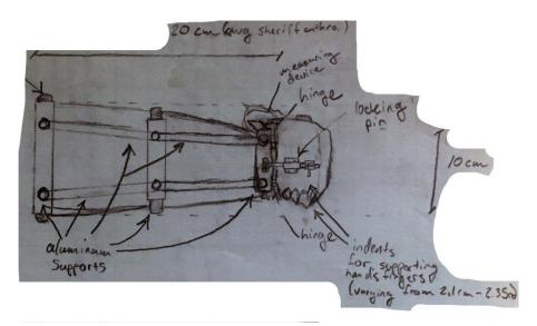
Figure 46: Exoskeleton D Drawings (Experimental)
