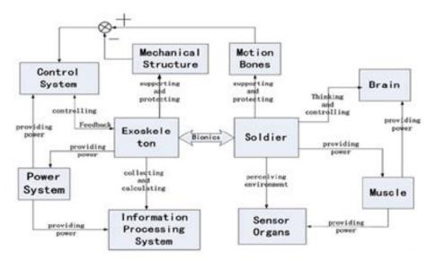
Figure 12: *The control principle of exoskeletons (Yuan, Wang, Ma, & Gong, 2014)* to a wall or stand (i.e., "grounded"), or to a wheelchair (Lo & Xie, 2012). This is adequate for applications where a limited and defined workspace is involved, or where a patient requires a
