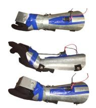
Figure 30: ARCTiC LawE Vrs. 2 (Top) Top down view - unactuated (Middle) Side view actuated (Bottom) Top down view - actuated)
