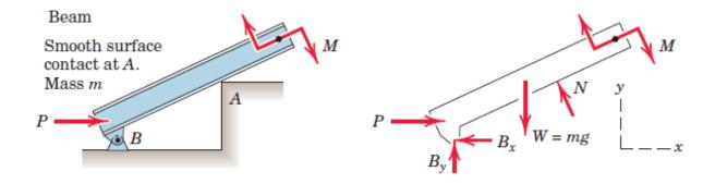
Figure 74: Sample Free Body Diagram
