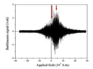
FIG. 4. Simulated BE signal for the hardened steel sample with a nominal case depth of 0.36 mm.
