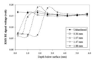
FIG. 2. Variation of the rms BE signal voltage with depth for the unhardened and surface-hardened samples with different case depths.
