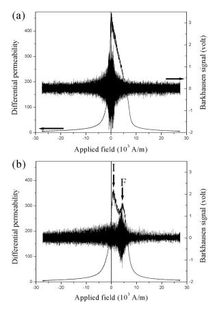
FIG. 1. Plots of the differential permeability and BE signal as a function of applied field for the (a) unhardened sample, and (b) surface hardened sample with a nominal case depth of 0.38 mm.
