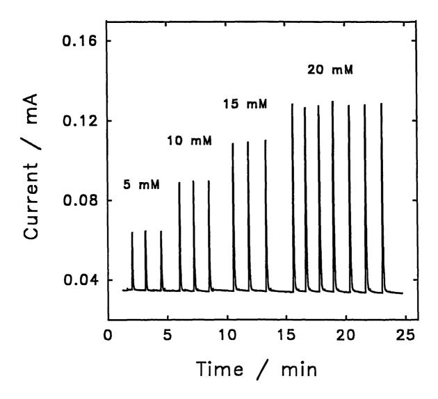
Figure 1.5. Representative flow-injection detection peaks for ethylamine at an anodized eutectic-phase Ag-Pb alloy electrode in 0.1 M carbonate buffer (pH 10). Carrier phase: 0.1 M carbonate buffer, 1.0 mL min<sup>-1</sup>. Potential: 0.90 V vs. SCE. Sample loop: 50  $\mu$ L. Ethylamine concentrations: given in figure.
