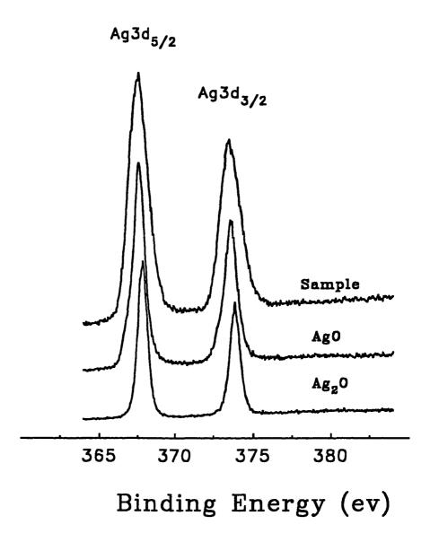
Figure 1.7. X-ray photon spectra showing Ag 3d<sub>5/2</sub> peaks for specified samples. Samples: (bottom) Ag<sub>2</sub>O film on Ag plate anodized at 0.3 V for 10 min in 0.1 M NaOH; (middle) AgO film on Ag plate anodized at 0.6 V for 10 min in 0.1 M NaOH; (top) oxide film on 1:20 (wt:wt) Ag-Pb alloy anodized at 0.9 V for 30 min in 0.1 M carbonate buffer (pH 10).
