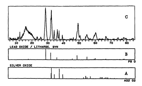
Figure 1.6. X-ray diffraction spectra: (A) silver oxide (AgO); (B) litharge (PbO); and (C) surface of 1:5 (wt:wt) Ag-Pb alloy electrode anodized in 0.1 M carbonate buffer (pH 10) at 0.90 V for 12 hrs.
