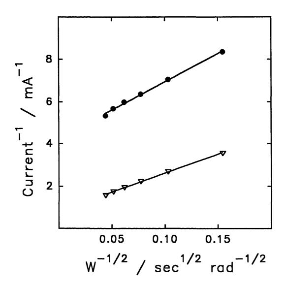
Figure 3.5. Representative Koutecky-Levich plots for 2.00 mM alanine in 1.0 M carbonate buffer (pH 10). Temperature (°C): (●) 10, (∇) 40.
