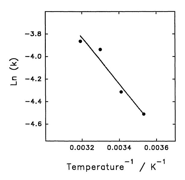
Figure 3.6. Arrhenius plot for 2.56 mM ethylamine in 1.0 M carbonate buffer (pH 10).
