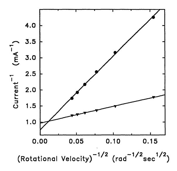
Figure 2.2. Koutecky-Levich plots for voltammetric peak responses for (∇) 2.0 mM NH<sub>4</sub>HCO<sub>3</sub> and (●) 2.0 mM ethylamine in 0.1 M carbonate buffer (pH 10). Scan rate: 2.0 V min<sup>-1</sup>.
