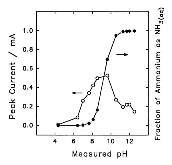
Figure 2.3. Correlation of voltammetric peak response and calculated concentration of NH<sub>3</sub>(aq) as a function of pH. Buffer: 50 mM NaH<sub>2</sub>PO<sub>4</sub> adjusted to pH by NaOH. Scan rate: 2.0 V min<sup>-1</sup>. Rotational velocity: 168 rad s<sup>-1</sup>.
