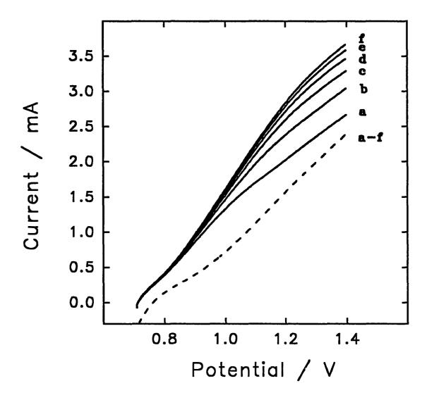
Figure 2.1. Voltammetric responses (pos. scan) for (NH<sub>4</sub>)SO<sub>4</sub> at an anodized eutectic-phase Ag-Pb alloy disk electrode as a function of rotation speed in 0.1 M carbonate buffer (pH 10). Scan rate: 2.0 V min<sup>-1</sup>. Concentration of (NH<sub>4</sub>)<sub>2</sub>SO<sub>4</sub> (mM): (- - - -) 0, (———) 1.0. Rotational velocity (rad s<sup>-1</sup>): (a) 42, (b) 94, (c) 168, (d) 262, (e) 377, (f) 513.
