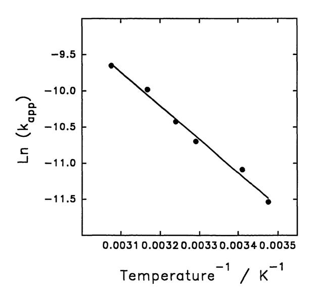
Figure 3.9. Arrhenius plot for oxidation of NH<sub>3</sub>(aq) in flow-through reactor.
