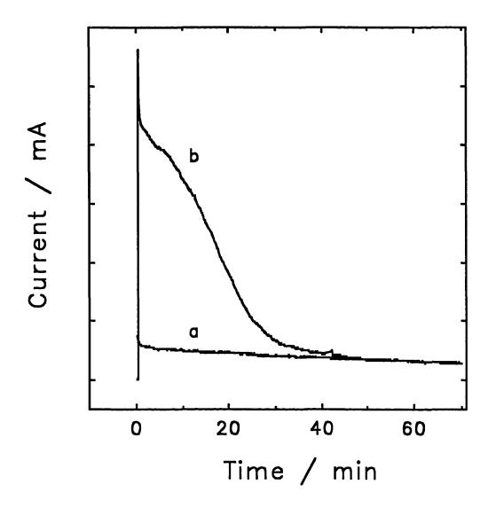
Figure 2.5. Current-time profiles for the exhaustive electrolysis of ethylamine in stirred 0.1 M carbonate buffer (pH 10). Wire electrode (ca. 9 cm<sup>2</sup>): anodized eutectic phase of Ag-Pb alloy. Potential: 1.0 V vs. SCE. Curves: (a) residual, (b) 17.5 mM (NH<sub>4</sub>)<sub>2</sub>SO<sub>4</sub>.
