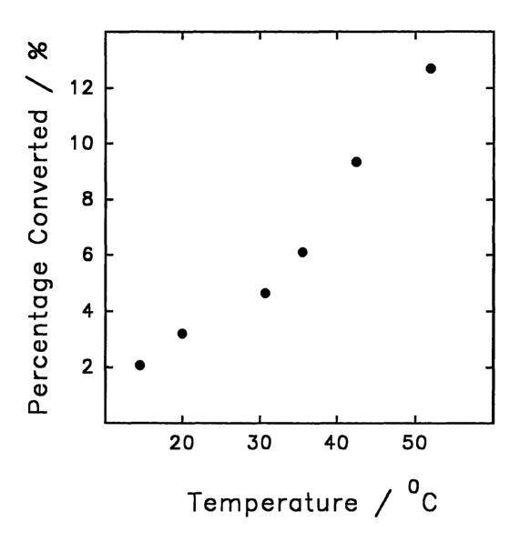
Figure 3.8. Percent conversion of total ammonia to nitrate ion in the flow-through reactor as a function of temperature. Flow rate:  $8.2 \times 10^{-3}$  cm<sup>3</sup> s<sup>-1</sup> (0.50 mL min<sup>-1</sup>).
