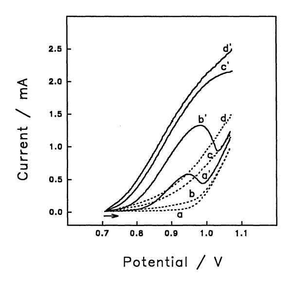
Figure 1.1. Voltammetric response (pos. scan) for ethylamine at various electrodeposited Ag-Pb oxide rotated disk electrodes in carbonate buffer (pH 10). Scan rate: 2.0 V min<sup>-1</sup>. Rotation speed: 3600 rev min<sup>-1</sup>. Film-deposition solution: 40 μM Pb(II) with variable Ag(I) in carbonate buffer (pH 10); [Ag(I)]/[Pb(II)]: (a,a') 1/40, (b,b') 1/10, (c,c') 1/4, (d,d') 1/2. Ethylamine concentration (mM): (- - - -) 0, (———) 3.9.
