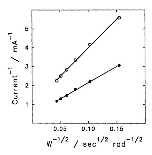
Figure 3.4. Representative Koutecky-Levich plots for 2.56 mM ethylamine in 1.0 M carbonate buffer (pH 10). Temperature (°C): (O) 10, ( • ) 40.
