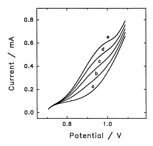
Figure 1.2. Voltammetric response (pos. scan) at an anodized eutectic-phase Ag-Pb alloy RDE as a function of ethylamine concentration in carbonate buffer (pH 10). Scan rate: 2.0 V min<sup>-1</sup>. Rotation speed: 1600 rev min<sup>-1</sup>. Ethylamine concentration (mM): (a) 0, (b) 0.5, (c) 1.0, (d) 1.5, (e) 2.0.
