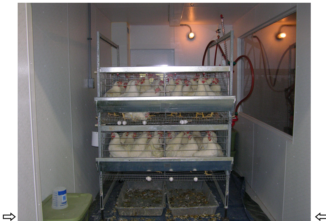
Figure 2. Inside a room outfitted to house 80 laying hens at the Animal Emissions Laboratory at Iowa State University.
