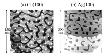
FIG. 1. Wormlike vacancy nanoclusters formed after deposition of  $\sim 0.6$  ml of film on the surfaces of (a) Cu(100); (b) Ag(100).
