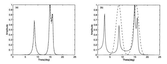
Figure 3. (a) Comparison of angular (spatial) spectra (solid curve) of the x-scan data at incident angles of  $8.5^{\circ}$ (first sharp peak) and  $15.5^{\circ}$ (second two peaks) in the previous figure and a direct calculation (dashed curve) using Eq. (4); (b) a physical illustration of Eq. (4).
