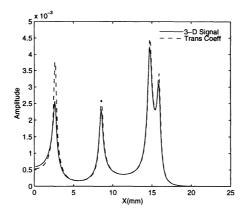
Figure 5. Comparison of plane-wave transmission coefficient (dashed curve) and reconstructed transmission coefficient from 3-D voltage calculation when the object distance is 30 mm.
