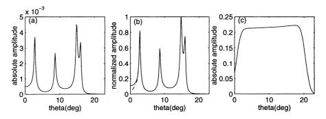
Figure 4. (a) Plane-wave transmission coefficient (solid curve) and 2-D synthetic reconstructed signal normalized by window (dashed curve); (b) Transmission coefficient (solid line) and the 2-D synthesized transmitted signal not normalized by window at right; (c) Window produced by summing the angular spectra of several incident angles with no plate.
