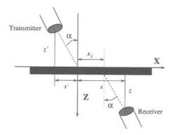
Figure 1. Schematic diagram of experimental transmission setup.
