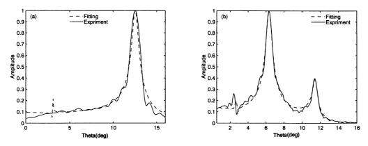
Figure 7. The reconstructed transmission coefficient (solid curve) of a biaxial graphite epoxy laminate and best fit results (dashed curve). (a) f=0.41MHz, (b) f=1.1MHz.
