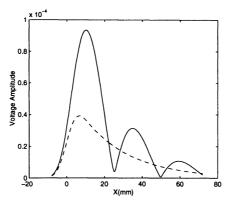
Figure 2. Transmitted signal calculated from Eq. (3) (with the plane-wave transmission coefficient) for a Plexiglas plate at an incident angle of  $15^{\circ}$  (solid curve) and  $8.5^{\circ}$  (dashed curve) as a function of scan coordinate x.
