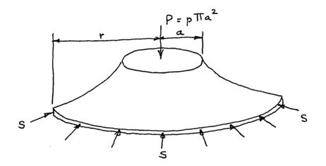
Because of symmetry, the normal stress S is assumed to be constant around the cut circle as shown. The slope at which the resultant stress S acts is assumed to be equal to the slope of the middle surface of the shell in the radial direction at that point. This slope may be represented by
