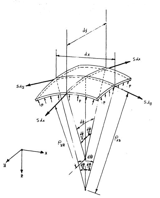
ASSUME THE RESULTANT TENSILE FORCES ON THE CUT SECTIONS ARE TANGENT TO THE TRACES OF THE SURFACE IN THE XZ AND YZ PLANES AS SHOWN.
