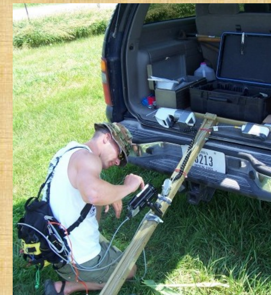
Fig. 2. A view from the Crop Circle and GreenSeeker canopy sensor's perspective. Includes 5 N fertilizer rates (0-240 kg N ha -1 ) in CC and CS crop rotations. The distance to canopy is 90 cm at the V10 corn growth stage.
