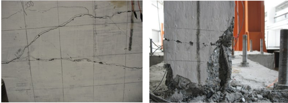
Figure 11. Main crack and concrete spall of W1.[33]
