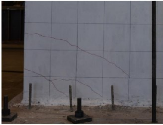
(a) Cracks resulted from threaded insert
