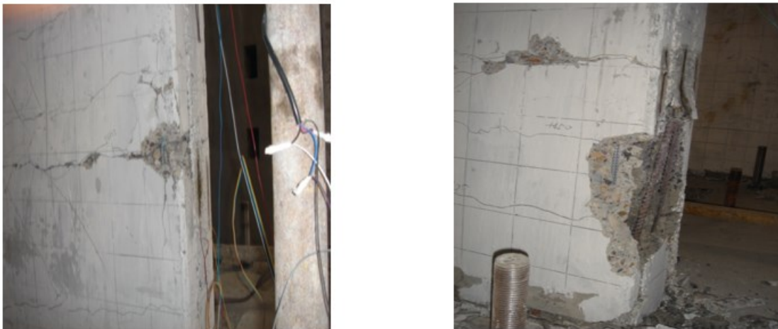
Figure 13. Main crack and concrete spall of W3.[33]
