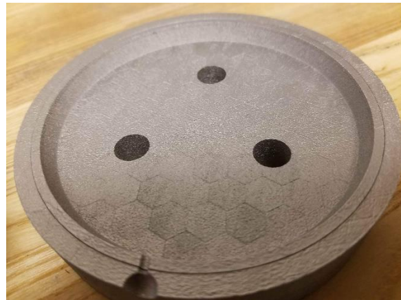
Figure 31: Part fabricated with hex infill pattern visible
