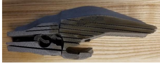
Figure 14: Reducing post-processing by utilizing breakable supports
