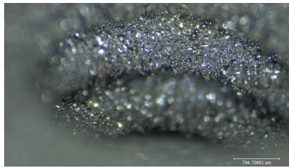
Figure 20: Microscope image of 1/4-20 thread printed horizontally
