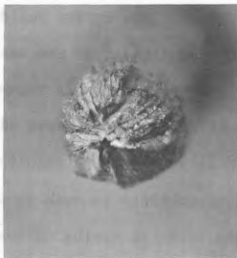
Figure 11. Example of a typical strained tensile specimen illustrating nearly 100% reduction in area X15
