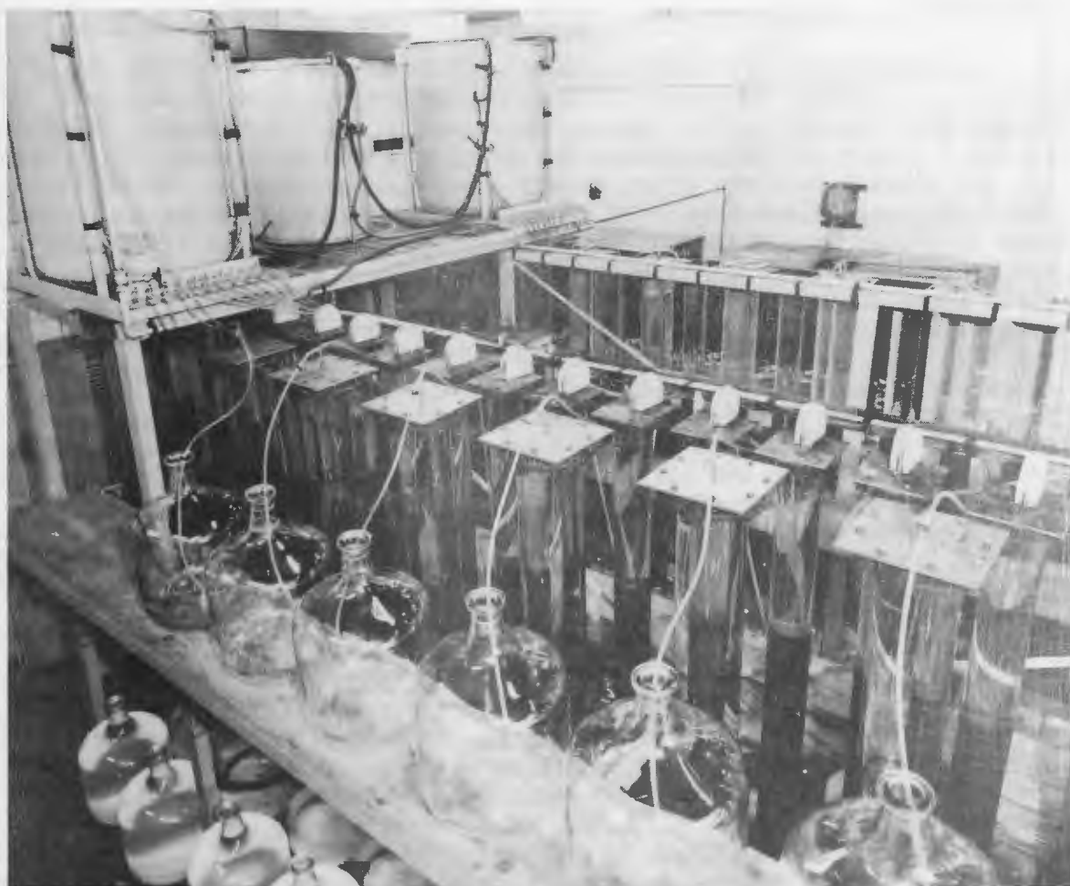
Figure 2 - Pilot-plant for separating rare earths.
