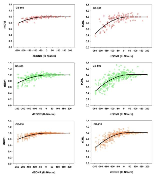
**Figure 1.** Relative canopy index values and regression models as related to the differential from the economic optimum N rate (dEONR) for the GreenSeeker 505 (GS-505), GreenSeeker 506 (GS-506), and Crop Circle ACS-210 (CC-210) active sensors.
