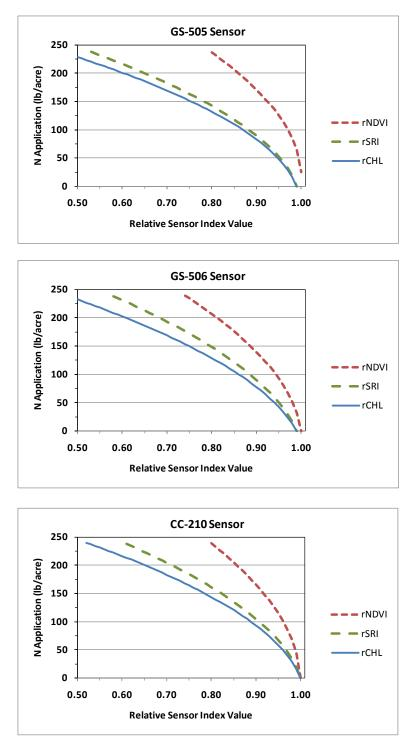
**Figure 2**. Nitrogen rate application prescriptions derived from the calibration models for the relative canopy indices from the GreenSeeker 505 (GS-505), GreenSeeker 506 (GS-506), and Crop Circle ACS-210 (CC-210) active sensors.
