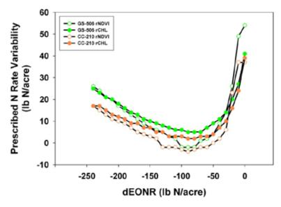
**Figure 3.** Sensor prescribed N rate variability across deficit differential economic optimum N rates (dEONR) for relative canopy indices from the GreenSeeker 506 (GS-506) and Crop Circle ACS-210 (CC-210) active sensors.
