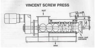
Figure 1. Vincent screw press manure solids separator.
