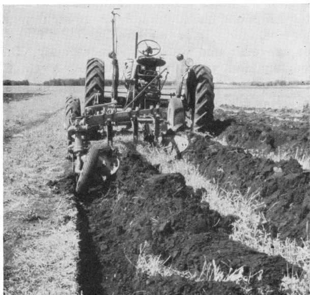
Ridge plowing with 4-bottom plow that has the 2 center bottoms removed.
