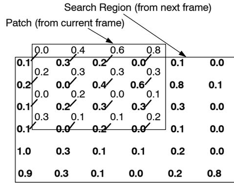
Figure 2. Process of calculating an error matrix (Err). The patch was shift over the search region. For the position shown above  $Err_{1,1} = |(0.0 - 0.1)| + |(0.4 - 0.3)| + \dots + |(0.2 - 0.0)| = 3.3$ .
