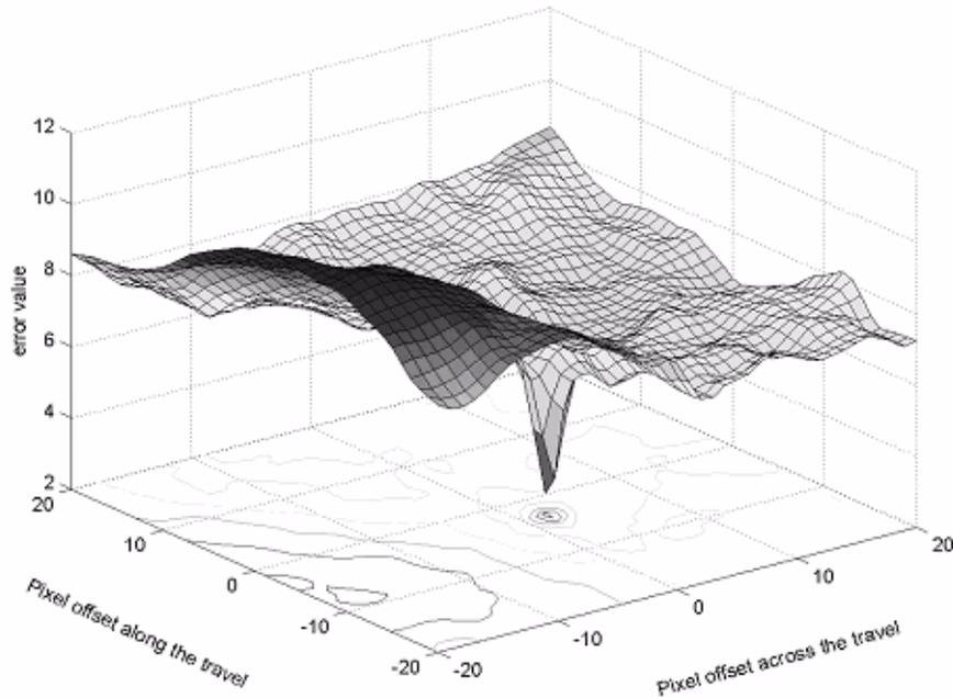
Figure 3. Example of an error surface and its contour for a typical patch matching. The minimum error value must be significantly different from the mean error to be accepted as a valid match.
