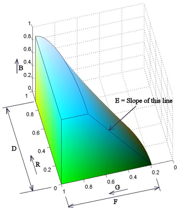
**Figure 4.** The truncated ellipsoidal decision surface in RGB color space used to segment vegetation from background. A pixel with RGB intensities inside the ellipsoid is considered a plant pixel. Parameter values used to segment plant from background were:  $D = 0.9$ ,  $E = -0.57$ , and  $F = 0.81$ .
