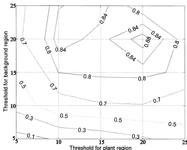
Figure 6. Contour plot of  $R^2$  for different combinations of plant and background region thresholds. Thresholds between 10 and 20 for the plant region and thresholds between 15 and 25 for the background region produced  $R^2 > 0.8$ .
