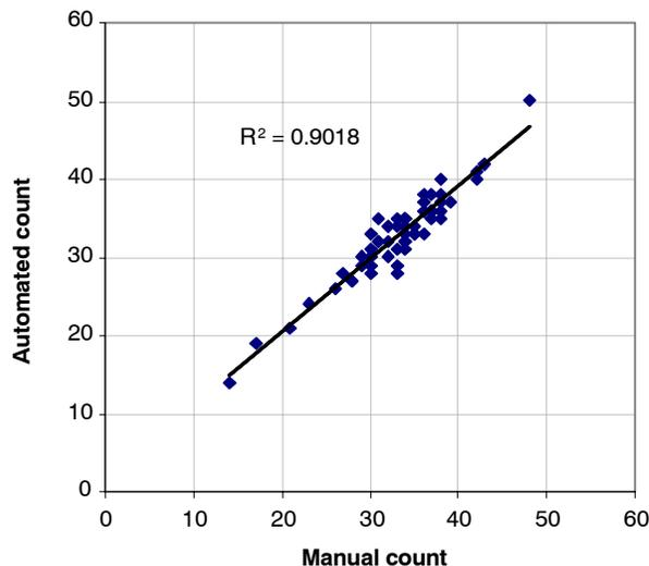
Figure 5. Regression of system-estimated counts onto manual counts for 60 experimental units. The regression had an  $R^2$  of 0.9018 and an RMSE of 1.8 plants.
