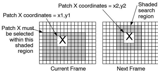
Figure 1. For image sequencing, an image patch (X) in the current frame was shifted in a search region in the next frame to find the best match. The difference in coordinates of the patch matched to the second frame gives the amount of shift from the current frame to the next frame.
