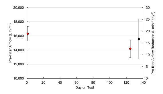
Figure 1 Average pre-filter airflow change from pre-test to post-test, red circles, error bars represent 1 standard deviation of all sow farms observed. On the secondary Y axis the average pre-filter airflow reduction per day, black circle, the error bars represent one standard deviation of all sow farms observed. Note the days on the airflow reduction per day are arbitrary on this graph.
