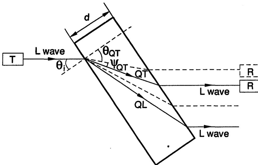
Figure 3.2: Oblique incidence of sound wave in an orthotropic plate submerged in water
