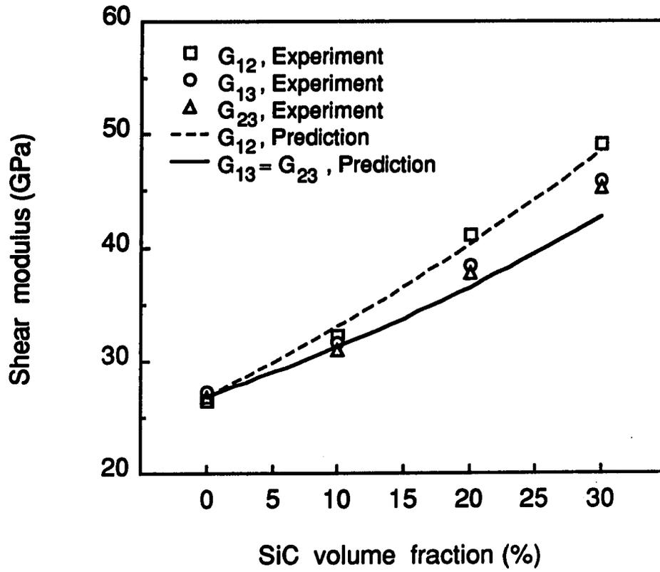
Figure 6.3: Comparison of predicted shear moduli  $G_{12}$  ( $= C_{66}$ ),  $G_{13}$  ( $= C_{55}$ ) and  $G_{23}$  ( $= C_{44}$ ) with experimental results (7091 Al/SiC<sub>p</sub>)
