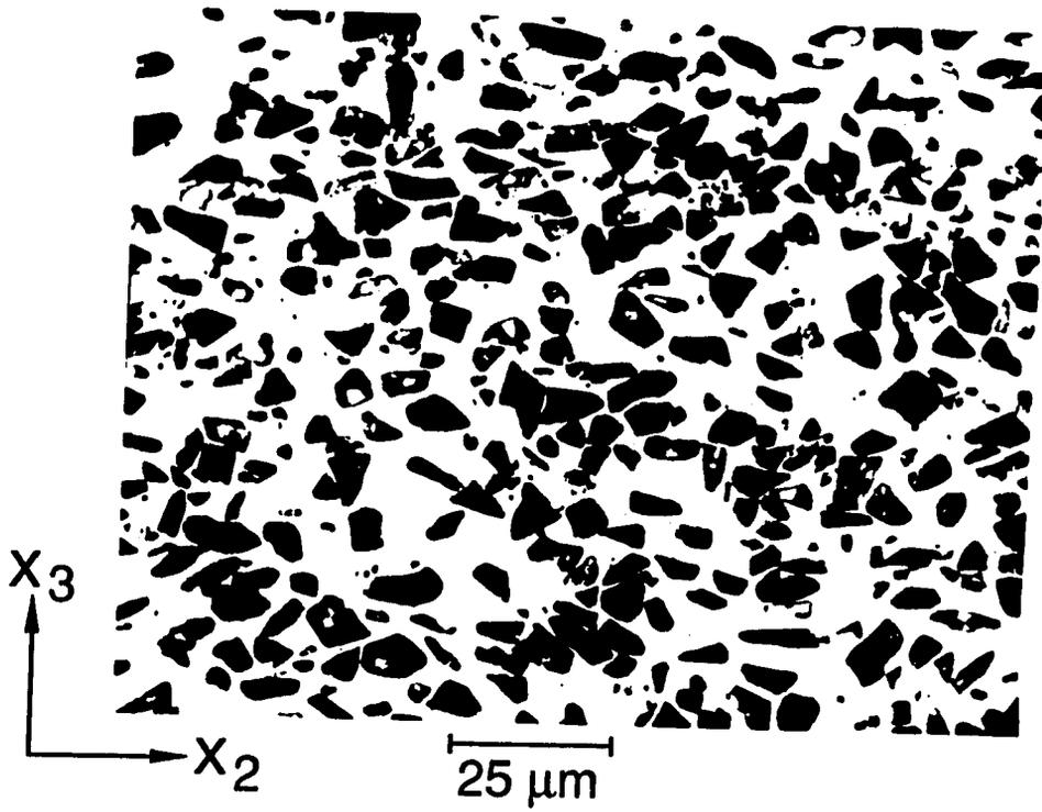
Figure 5.3: Photomicrograph taken on the  $x_2$ - $x_3$  plane of 30% SiC<sub>p</sub>/7091 Al (PE-2665)
