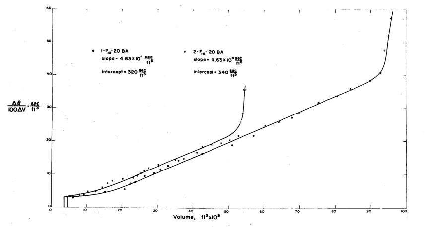
Figure 17. Plots of  $\Delta \Theta / \Delta V$  versus V for constant pressure filtrations
