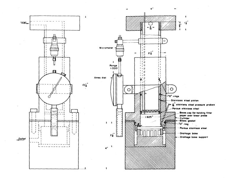
effect of piston and drainage-base septum resistances. Mechanical loading was done by direct addition of weights to the piston. The solids compressive pressure was calculated from these weights and the piston area  $(2.0742 \text{ in}^2)$ .
