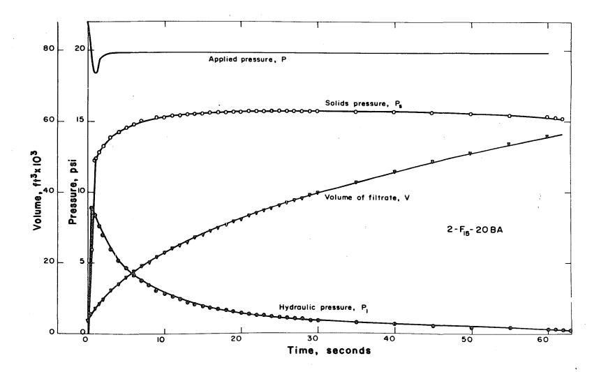
Figure 13. Volume of filtrate V, applied pressure P, solids pressure  $P_8$ , and hydraulic pressure  $P_1$ , as functions of time for a constant pressure filtration
