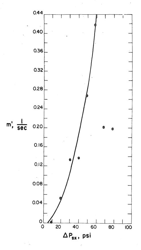
pressure is increasing continuously, there must be a total solids pressure increment of at least 5 psi before there is any change in porosity. Consequently assumption 1 is not valid for calcium carbonate. The time lag is at least the time necessary for  $P_{sx}$  to change 5 psi.
