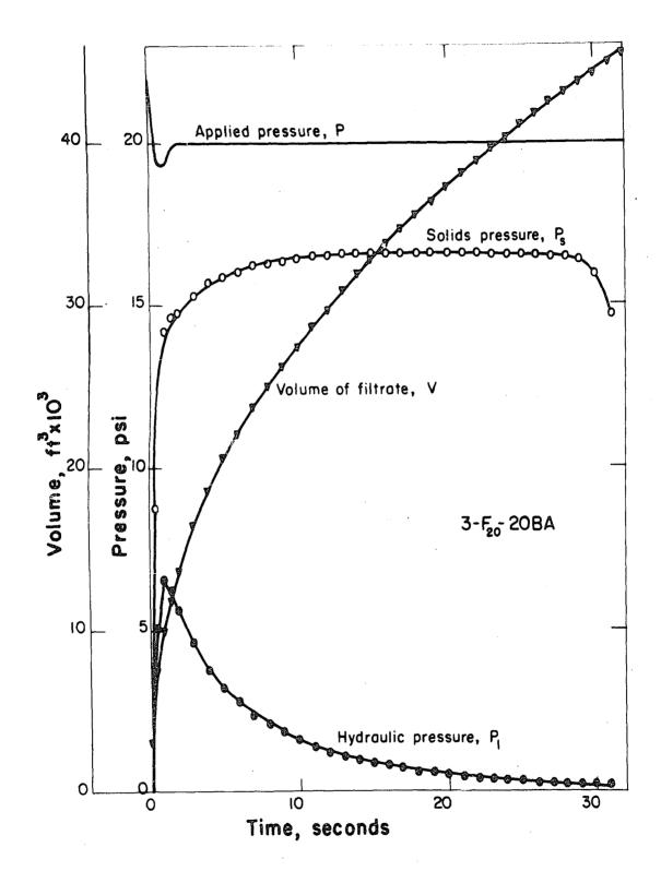
Figure 14. Volume of filtrate V, applied pressure P, solids pressure  $P_s$ , and hydraulic pressure  $P_l$ , as functions of time for a constant pressure filtration
