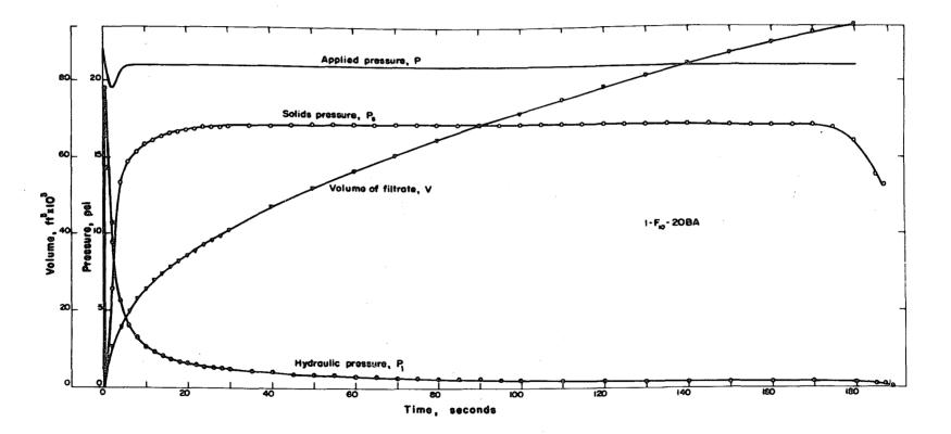
Figure 12. Volume of filtrate V, applied pressure P, solids pressure  $P_s$ , and hydraulic pressure  $P_1$ , as functions of time for a constant pressure filtration
