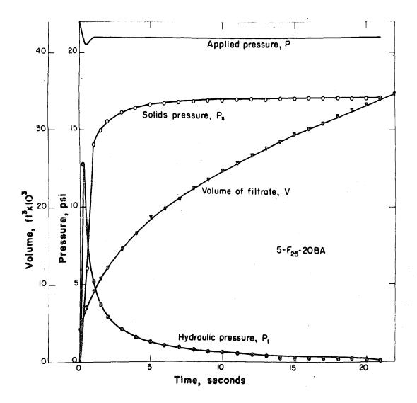
Figure 15. Volume of filtrate V, applied pressure P, solids pressure  $P_s$ , and hydraulic pressure  $P_l$ , as functions of time for a constant pressure filtration
