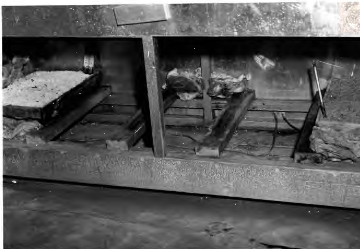
Fig. III. The aluminum propagating cabinet with the three middle flats removed to show arrangement of the heating cable at the bottom.
