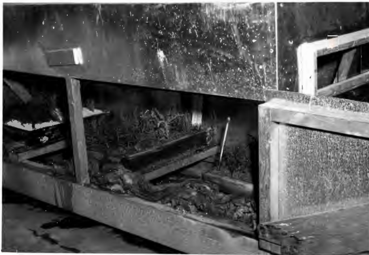
Fig. II. The aluminum propagating cabinet, showing the ventilation window at one end. The two doors are opened and the second and fourth flat are removed to give a clear view of the interior.
