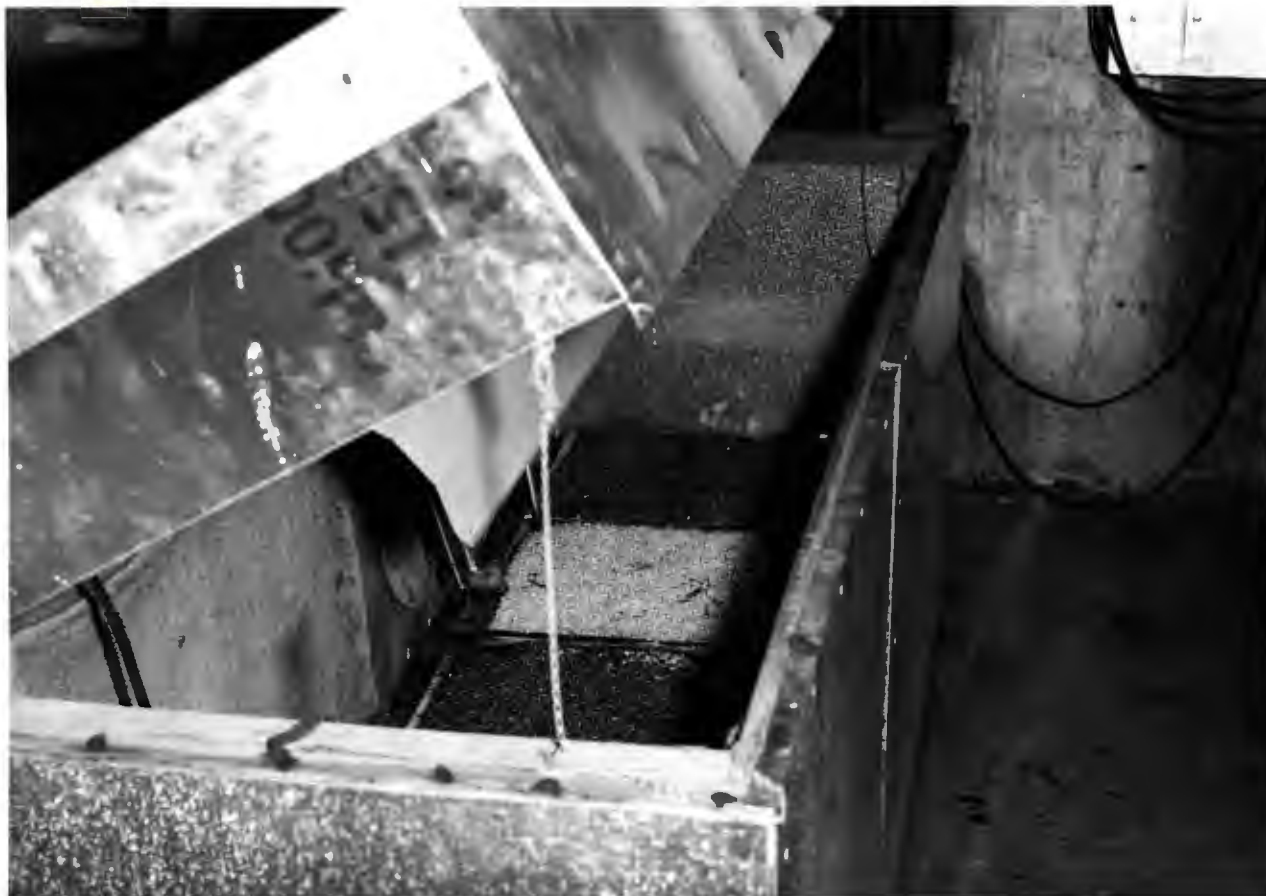
Fig. I. The aluminum propagating cabinet, showing the hinged cover and the arrangement of flats and psychrometer inside of the cabinet.
