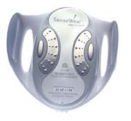
temperature, near body ambient temperature, heat flux, galvanic skin response, and motion via a 2-axial accelerometer. It has a built-in thermostat based sensor to measure the surface temperature of the body. Near body ambient temperature measures the air temperature around the armband to reflect temperature changes in the environment. Heat flux measures the rate at which heat is dissipating
