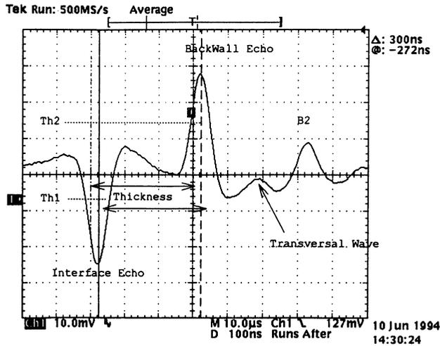
Figure 12. Multiple echo form of 1mm aluminum plate
