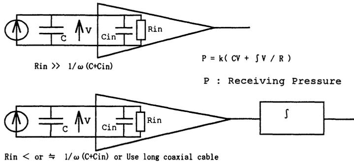
Figure 5. Two method for reproduction of receiving pressure
