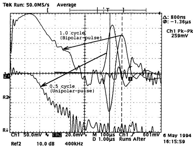
Figure 10. Received waveform of 0.5 and 1.0 cycle
