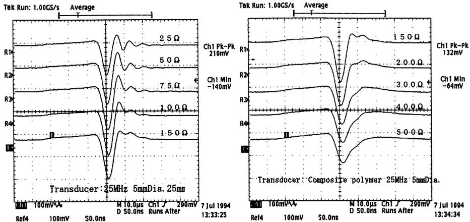
Figure 11. Waveform changes according to discharge resistor  $R_o$
