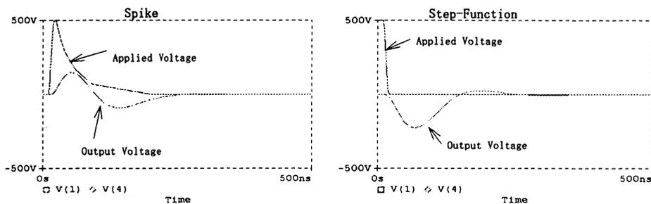
Figure 1. Analysis of spike- and step-function pulser by PSpice
