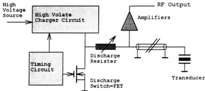
Figure 3. Simplified equivalent circuit of step-function pulser
