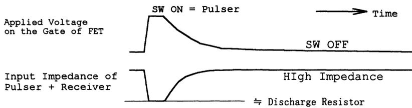
Figure 6. Input impedance
