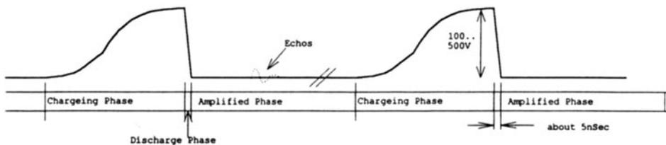
Figure 4. Electrical waveform at drain of FET
