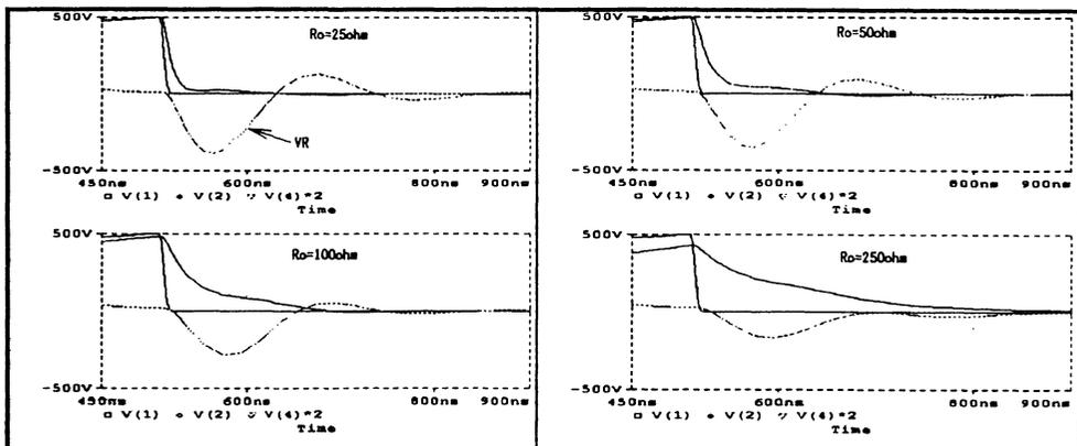
Figure 2. Waveform vs. discharge resistor
