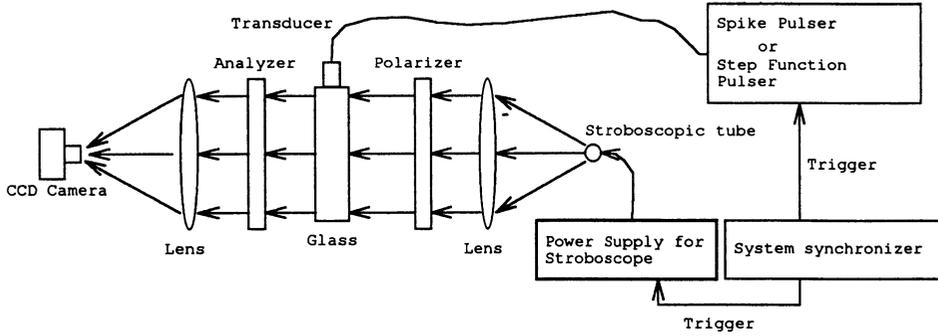
Figure 7. Block diagram of ultrasonic visualization system
