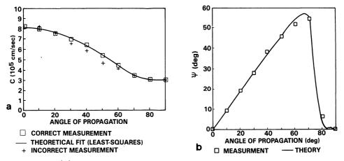
Figure 4. (a) Quasi-longitudinal phase velocity in 1-2 plane of unidirectional AS4/3501-6 prepreg composite. (b) Group velocity deviation angle for same material.
