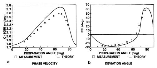
Figure 6. (a) Quasi-shear phase velocity for 1-3 plane of unidirectional AS4/3501-6 material. (b) Group velocity deviation angle for 1-3 plane of same material.
