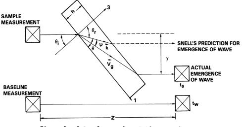
Figure 5. Setup for sample rotation experiment.
