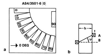
Figure 3. (a) Samples cut from AS4/3501-6 panel. (b) Group velocity vector deviation in off-axis samples.
