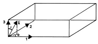
Figure 2. Laminate Coordinate System.
