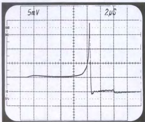
Figure 5. Oscillogram showing result of impulse surface pulse for aluminum-alloy block, Poisson's ratio equals 0.343, 6.3 cm thick and 17.8 cm in diameter. The breaking of a glass capillary 0.15 mm in diameter is the source. Electrostatic transducer is located 5.08 cm from source. Each division or abscissa equals 2\mu sec.
