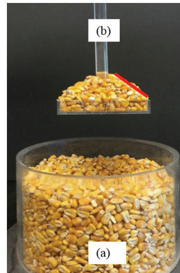
Figure 2. (left) Simple experiments for bucket-discharged AOR ( \alpha_{\text{bucket}} ) and (right) anchor-lifted AOR ( \alpha_{\text{anchor}} ) in which an anchor (b) was lifted to form an angle of repose (AOR) from a cylinder (a) loosely filled with corn.
