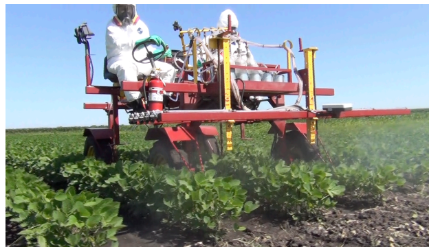
Figure 2. Self-propelled research sprayer applying treatments in Ames, IA.
