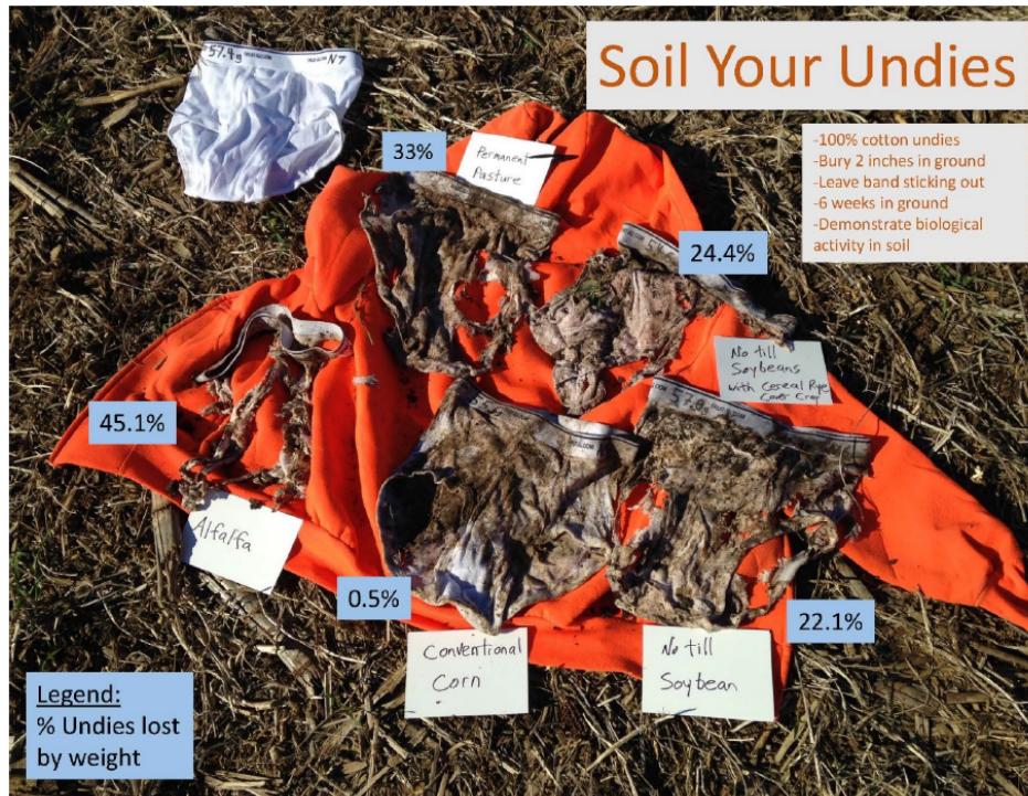
Figure 3. Soil your undies demonstration done by Neil Sass at Soil Survey Office in Waverly, IA. The percent mass of cotton left at the end of 6 weeks in (top and clockwise) perennial pasture, no-till soy with rye cover, no-till soybean, conventional corn, and alfalfa. Original cotton underwear shown in upper left.
