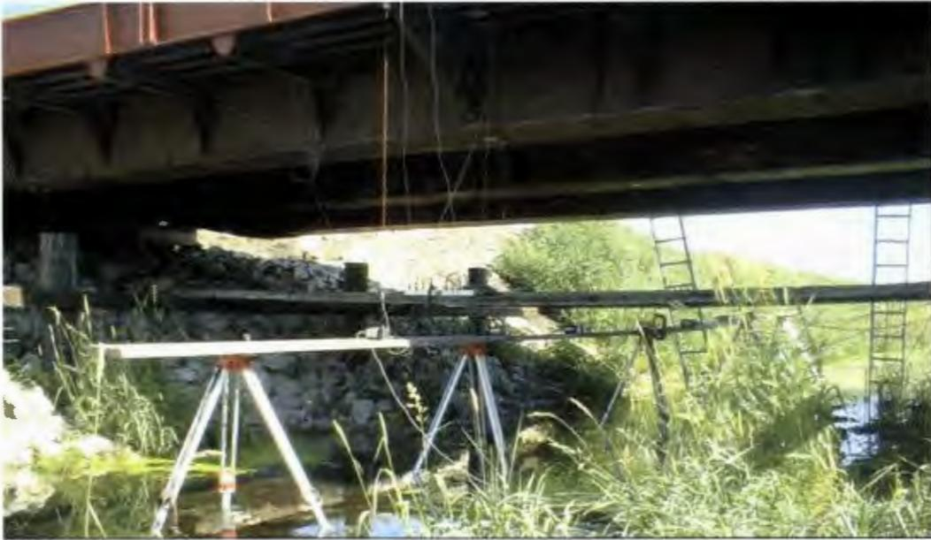
a. Installed deflection instrumentation on the WCB2
