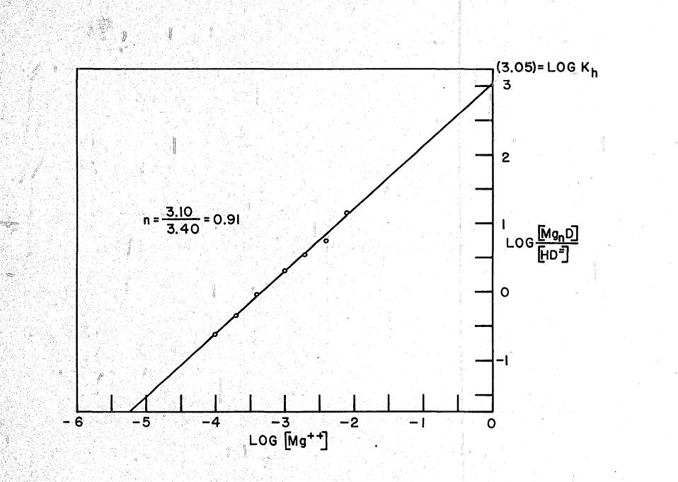
The extrapolation of the straight line gave the log of the apparent stability constant as 3.05 at pH 8.17. From this one would have 2.88 as the log of the stability constant at pH 8.0. Schwarzenbach's (22) value at pH 8 was 3.45. The agreement was not very good but it indicated that this work was in considerably greater agreement with the work of Schwarzenbach that it was with the work of the two American groups.
