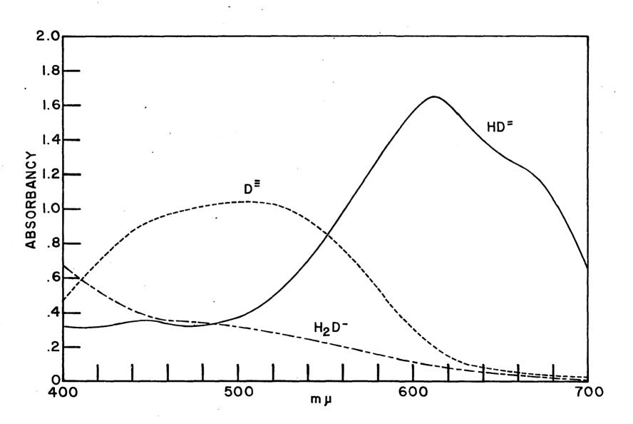
Figure 7. Absorption spectra of Eriochrome Black T and its calcium and magnesium derivatives at pH 10. Ionic strength;  $\mu = 0.100$
