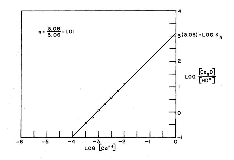
It was evident that calcium also formed a one to one compound with this indicator at pH 10. The logarithm of the apparent stability constant was found to be 3.05. It may be noted that this compound is weaker than the one formed between calcium and the p-cresol indicator.
