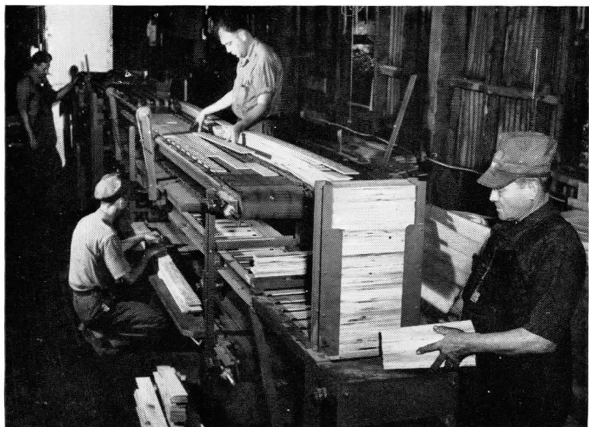
Fig. 2.—Feeding mechanism for continuous hydraulic glue press.
