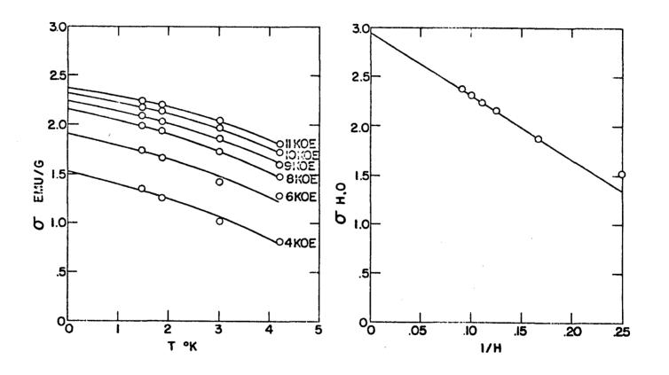
Figure 12.  $\sigma$  versus H for the single crystal of Ho-Y 1.0-99.0. The dashed curve represents the ideal paramagnetic behavior at 1.49 °K. See text.
