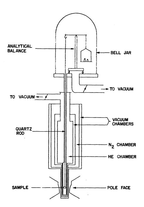
Figure 5. Detail of sample chamber used in magnetization measurements.
