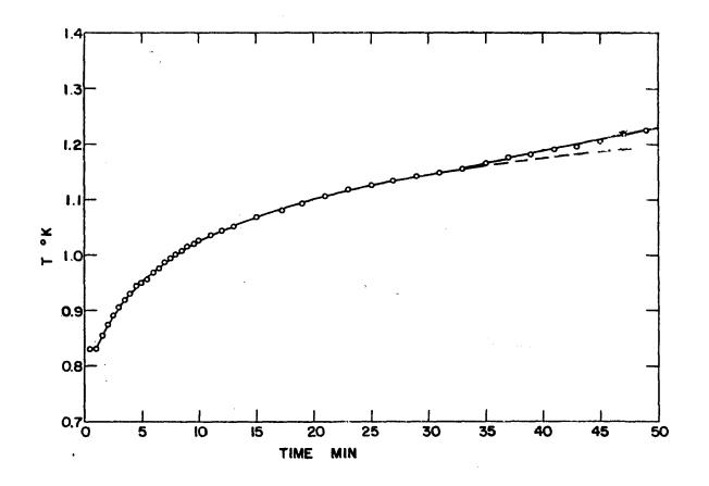
Figure 17. Warming curve after demagnetization of the alloy Ho-Y 1.0-99.0. The abscissa denotes time in minutes after the start of the demagnetization.
