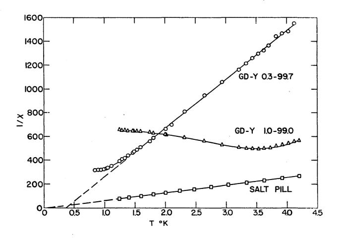
This means that a maximum occurs in the susceptibility at this temperature; such behavior is characteristic of a transition to the antiferromagnetic state below this temperature. There are insufficient experimental data above the transition temperature for a determination of the Curie constant and paramagnetic Curie temperature.
