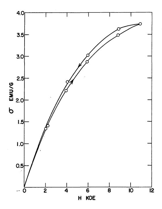
indicating the presence of ferromagnetic inclusions in the sample.
