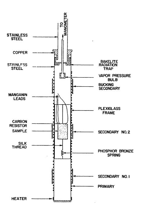
obtained during the same liquid helium run. Other susceptibility measurements for all samples were made with the sample centered in the sample tube with bakelite spacers. In each case the sample was brought to the temperature of the liquid helium bath by the introduction of helium exchange gas into the sample tube at a pressure of 50-100 microns. The radiation shield at the top of the sample tube prevented room temperature radiation from above from entering the sample chamber.
