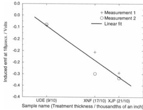
Figure 6. Pulse height variation with aluminized treatment thickness.
