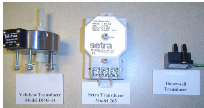
Figure 2.2. Three different transducers which input wind speed from pressure tubes and output a corresponding voltage
