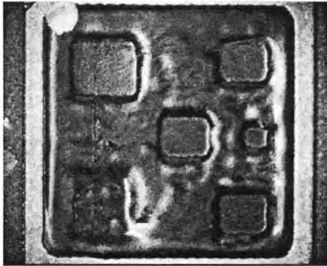
Figure 21. Device Coated with a Sample Encapsulant, 10X
