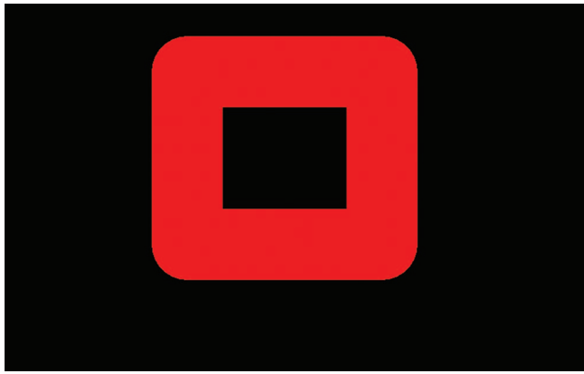
FIG. 6. Projected MATLAB image. The user can control the color, location, speed, and size of the shape using keyboard arrows and letters. The typical projected length scale is on the order of 10–100 \mu\text{m} after passing through the microscope objective.
