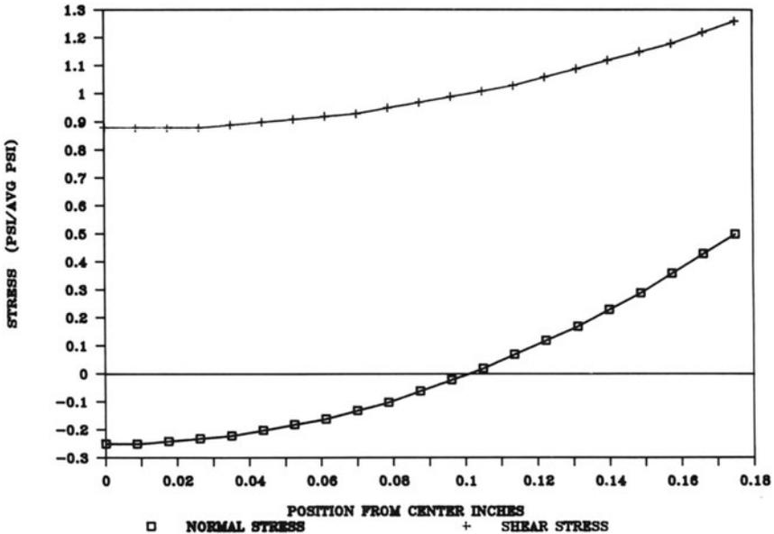
Fig. 4. Calculated Shear and Normal Stress Distribution in a .35 Inch Adhesive Lap Joint.
