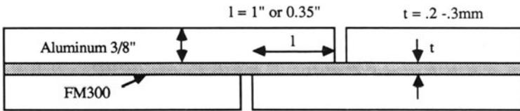
Fig. 3. Sample Geometry.
