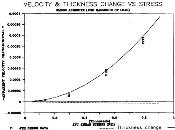
Fig. 9. Change of Shear Velocity in an Adhesive Joint and Adhesive Thickness as a Function of Shear Stress.
