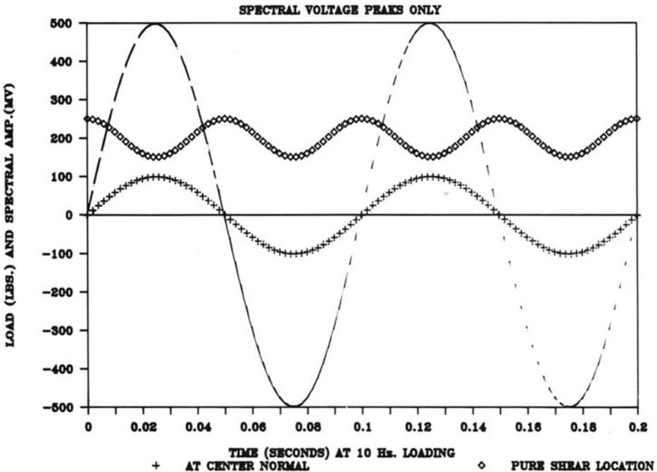
Fig. 7. Time Domain Outputs of the (a) Load, (b) First Harmonic, and (c) Second Harmonic of the Boxcar Amplifier.
