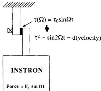
Fig. 1. Schematic Diagram of the Dynamic Acousto-Elastic Measurement in an Adhesive joint.
