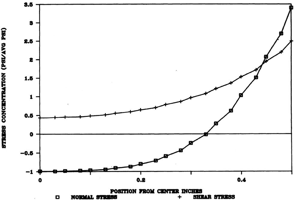
Fig. 2. Calculated Shear and Normal Stress Distribution in a 1" adhesive lap joint
