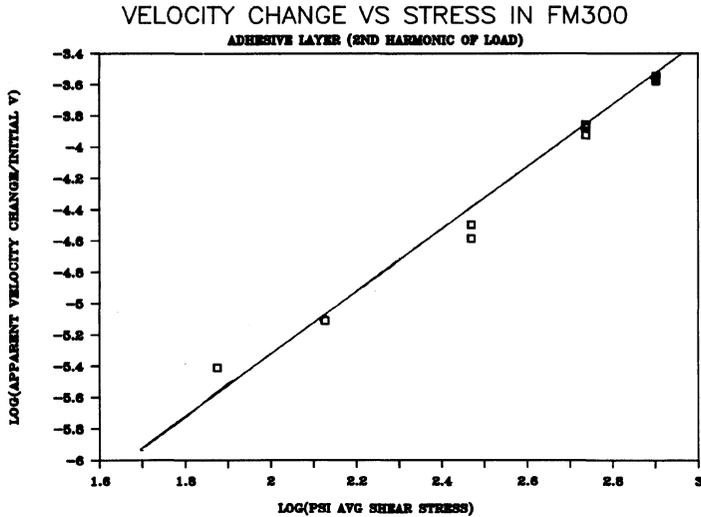
Fig. 10. Change of Shear Velocity in an Adhesive Joint as a Function of Shear Stress (Log Log Plot).
